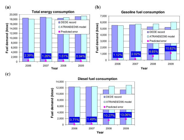
**Figure 4.** Validation of the energy demand model for fuel consumption in the years 2006–2009 for (**a**) all fuel types, (**b**) gasoline and (**c**) diesel fuels.
